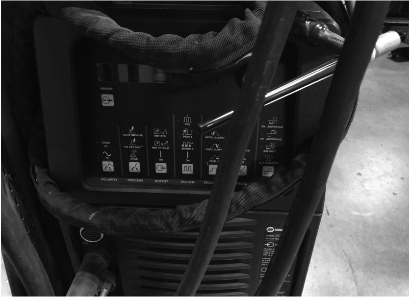
Figure I.3. Icons on a welding machine. A welding gun for GTAW rests on top of the machine.
