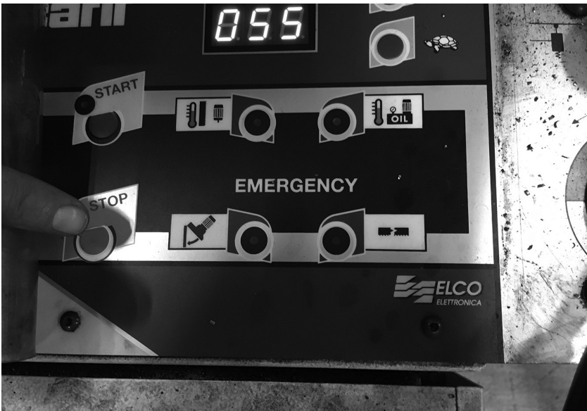
Figure I.4. Icons on a bandsaw. Note the turtle at the top right to indicate a slow speed.
